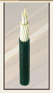
□ 600 / 1000 V-AUXILIARY CABLES (CONTROL CABLES) COPPER CONDUCTOR XLPE INSULATED PVC SHEATHED CABLES (CU / XLPE / PVC) SIZE: 4 SQMM
