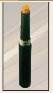
□ 600 / 1000 V - SINGLE CORE COPPER CONDUCTOR XLPE INSULATED ALUMINIUM WIRE ARMOURED **PVC SHEATHED CABLES**
