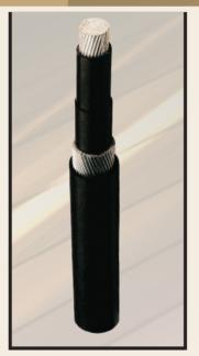
600 / 1000 V - SINGLE CORE ALUMINIUM CONDUCTOR PVC INSULATED ALUMINIUM WIRE ARMOURED
