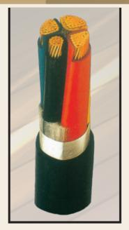
□ 600 / 1000 V - FOUR CORE WITH REDUCED NEUTRAL COPPER CONDUCTOR PVC INSULATED **PVC SHEATHED CABLES**
