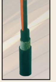
600 / 1000 V - TWO CORE COPPER CONDUCTOR PVC INSULATED STEEL WIRE ARMOURED **PVC SHEATHED CABLES**
