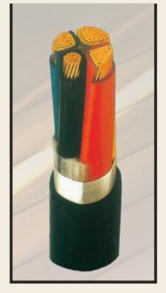
□ 600 / 1000 V - FOUR CORE WITH REDUCED NEUTRAL COPPER CONDUCTOR XLPE INSULATED **PVC SHEATHED CABLES**
