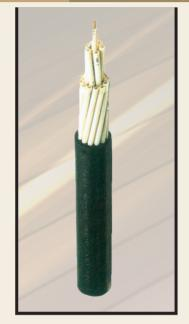
□ 600 / 1000 V-AUXILIARY CABLES (CONTROL CABLES) COPPER CONDUCTOR PVC INSULATED PVC SHEATHED CABLES (CU / PVC / PVC) SIZE: 1.5 SQMM
