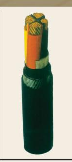
□ 600 / 1000 V - FOUR CORE WITH REDUCED NEUTRAL COPPER CONDUCTOR XLPE INSULATED STEEL WIRE ARMOURED PVC SHEATHED CABLES (CU/XLPE/PVC/SWA/PVC and CU/XLPE/SWA/PVC)
