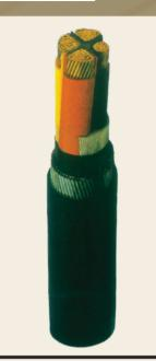
□ 600 / 1000 V - FOUR CORE WITH REDUCED NEUTRAL COPPER CONDUCTOR PVC INSULATED STEEL WIRE ARMOURED PVC SHEATHED CABLES
