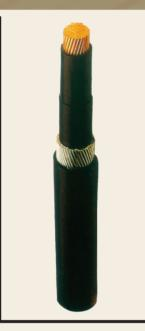
□ 600 / 1000 V - SINGLE CORE COPPER CONDUCTOR XLPE INSULATED ALUMINIUM WIRE ARMOURED **PVC SHEATHED CABLES**
