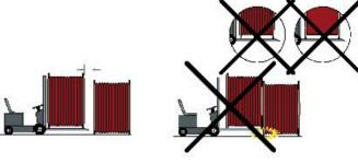
touch the ground. Paise the forks of the forklift at least 6 to 8 inches above ground. Insufficient clearance may cause the drum to be dragged on the ground and eventually damaged or dropped off the forks, especially if the ground surface is uneven.
