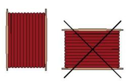
Always store and move the drum in an upright position. In no case, the drums be stored 'on the flat' that is with flange horizontal.
