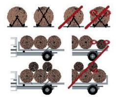
flanges with wires or ropes. To prevent movement of drums, a combination of wedges and transportation support should be used and tied down front and rear.
